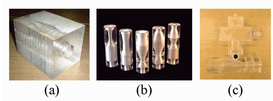
Fig. 1: Mechanical models of the human vocal cavity; (a) the plate-type model of vowel /a/; (b) cylinder-type models (from left, /i/, /e/, /a/, /o/ and /u/); and (c) a model for nasalized vowel /a/.
