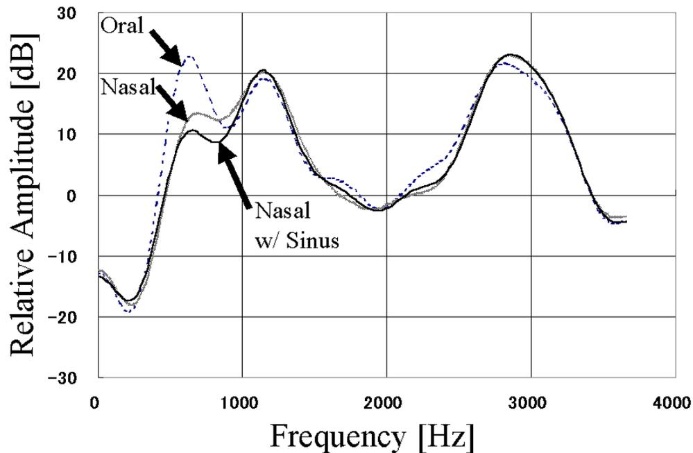
Fig. 2: Effect of the nasal cavity coupling on the spectral envelope (vowel /a/).
