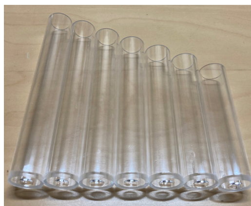
Fig. 2: Seven outer tubes of the sliding three-tube (S3T) model in this study.
