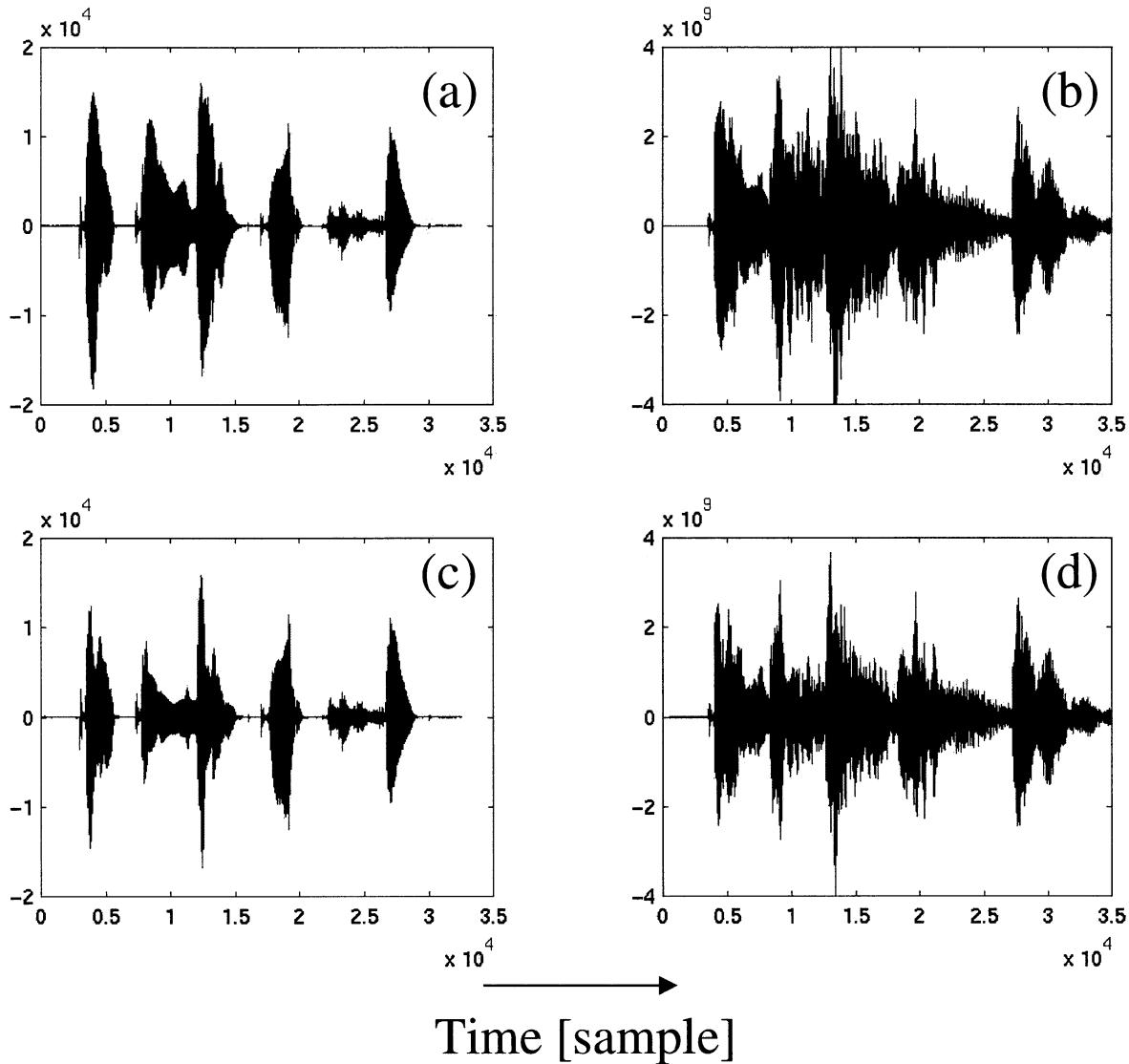
**Fig. 2** (a) Original waveform of a speech signal, (b) reverberant signal simulated by taking the convolution of the impulse response of a hall and the original signal, (c) suppressed signal of the original, and (d) reverberant signal of (c).
