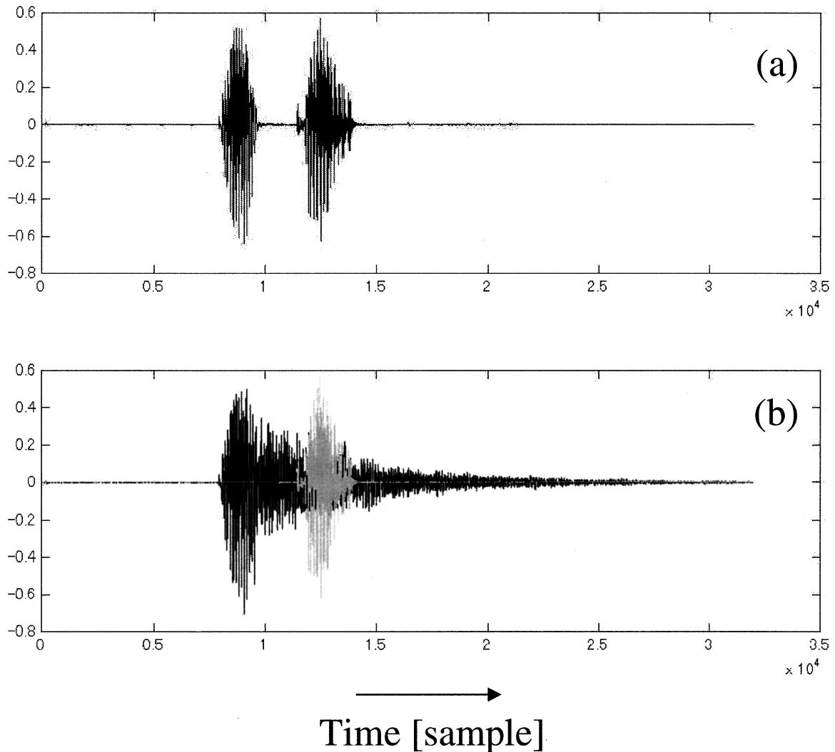
**Fig. 1** (a) Original waveform of a nonsense word /aka/, (b) simulated waveform obtained by taking the convolution of the impulse response of a hall and only the first vowel part of the original waveform. The /ka/ portion of the original waveform is shown with a lighter color in (b).
