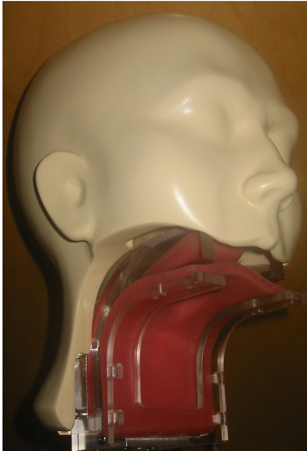
Fig. 8 Vocal-tract model with a gel-type tongue mounted in a head-shaped model.
