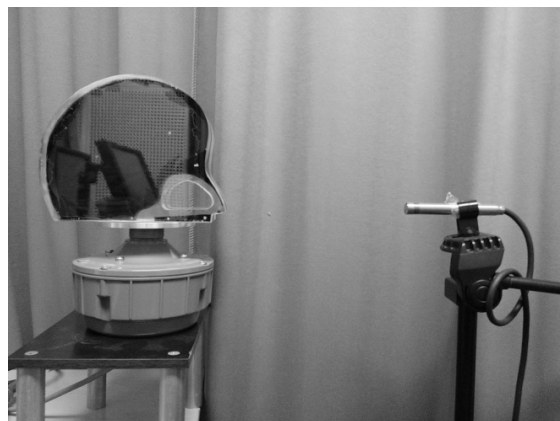
Figure 1: Measurement setup for nasal cavity model.
