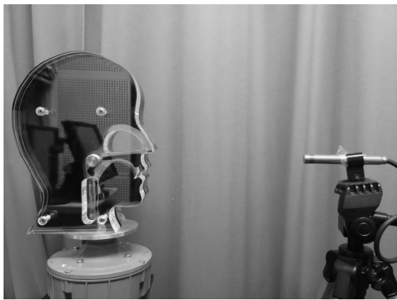
Figure 2: Measurement setup for head-shaped /a/ model.
