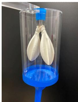
Fig. 1: Lung model with two small white balloons and a part of a big blue balloon as a diaphragm.
