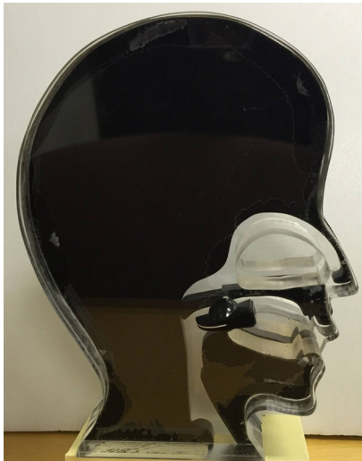
Fig. 3: Head-shape model with a nasal cavity. The degree of nasalization can be changed by rotating the valve [7].
