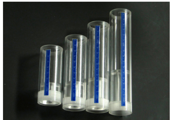
Fig. 4: Four acoustic tubes with different length (from [9]).
